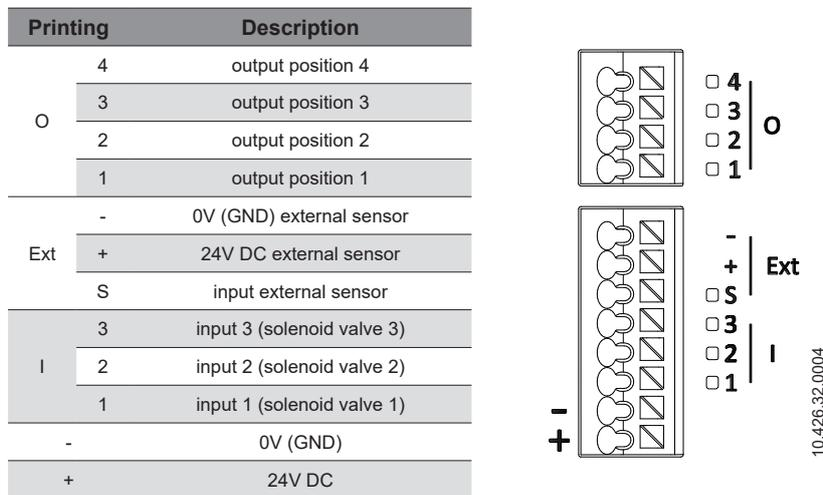
Wiring diagram digital 24 V DC communication for 1 solenoid valve and 3 outputs:
