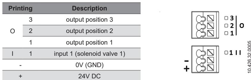
**5.7.2. Electrical installation with AS-interface communication**
